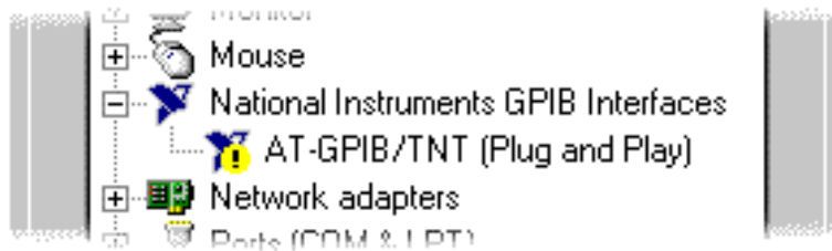
Figure 2-6. GPIB Interface That Is Not Working Properly
